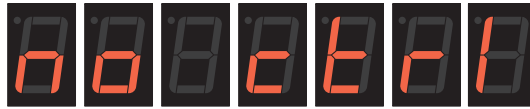
FIGURE 78. "No control" message will scroll when no valid radio signal is present
