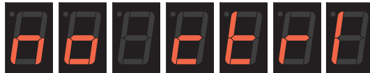
FIGURE 85. The “no control” message indicates that joystick is not centered at power up
